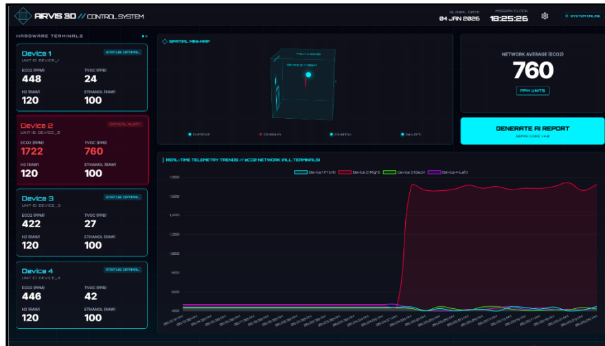
Fig. 5 Gas Leak Detection and visual alert
