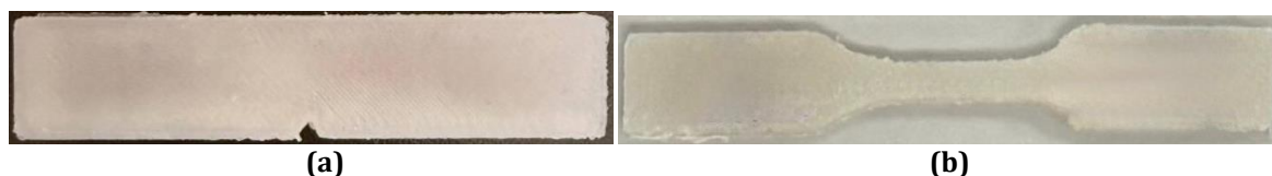
Fig 2.5 Printing specimens (a) ASTM D256 (Izod Impact Test); (b) ASTM D638 Type V (Tensile Test)
