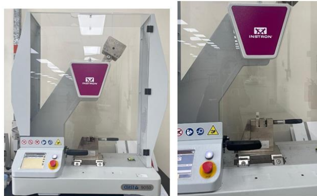
Fig 2.7 A pendulum impactor strike the specimen
