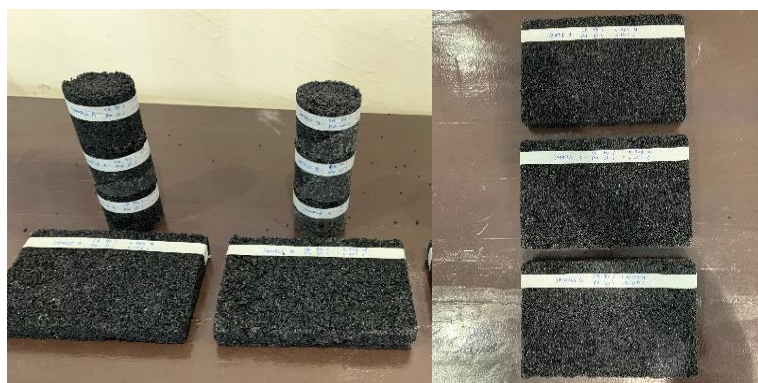
Fig 3. Sample Eco-Porous Paver
