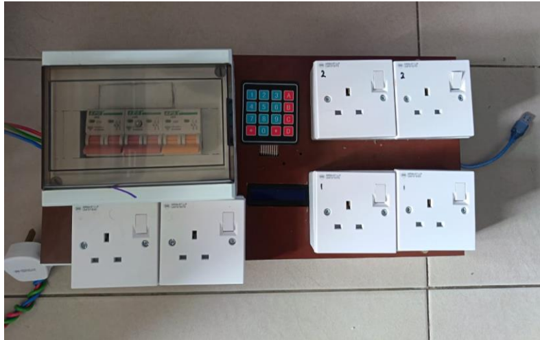
Fig. 5 Prototype of IoT-Enabled Automated Circuit Breaker
