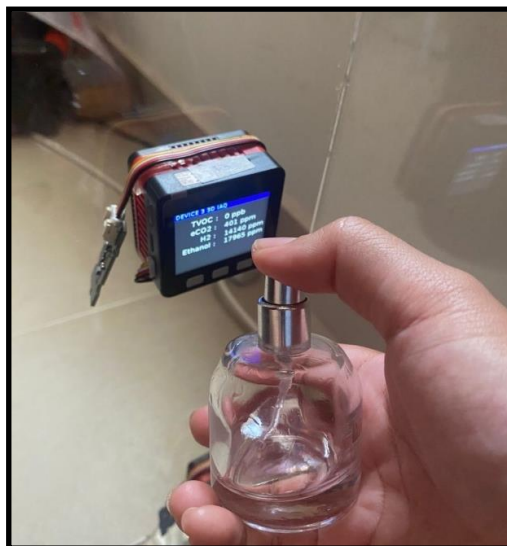
Fig.9 Simulated Gas Leakage Test Using Perfume Near Device 3
