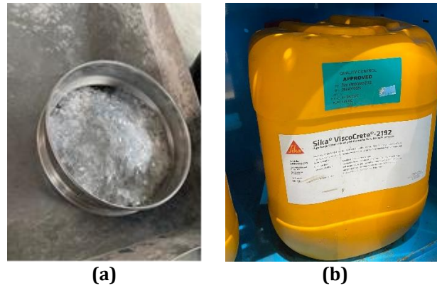
Fig. 1 (a) Sieving PET; (b) Sika® ViscoCrete®-2192
