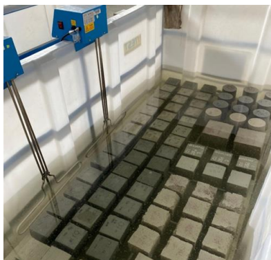
Fig. 2 Specimens submerged in curing tank
