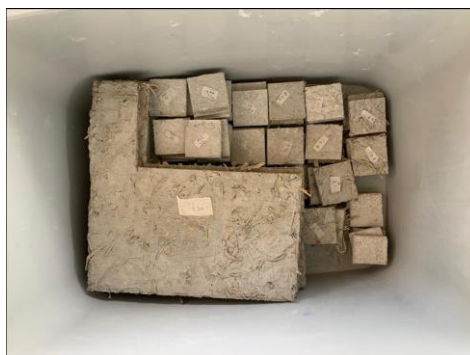
Figure 3: Cement board after cutting to size 50mm x 50mm.
