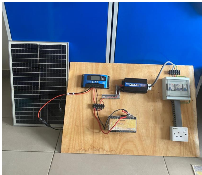
Figure 4 Hardware Prototype of solar application system
