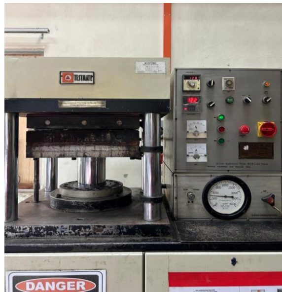
Figure 2 50-ton hydraulic hot press machine
