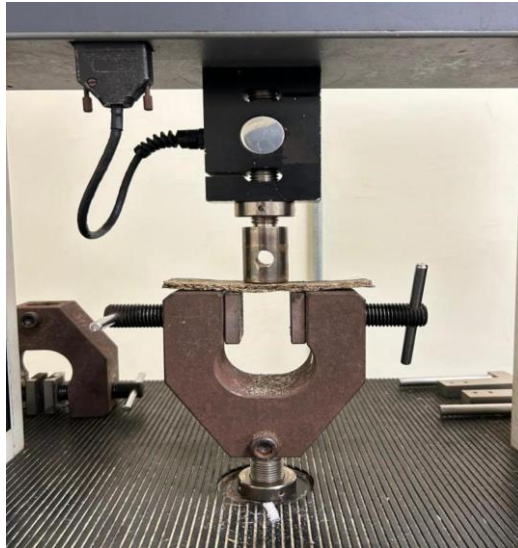
Figure 4 Bending (flexural) testing process
