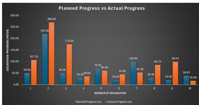
Fig 3 Planned Progress vs Actual Progress Graph for Gombak Tunnel
