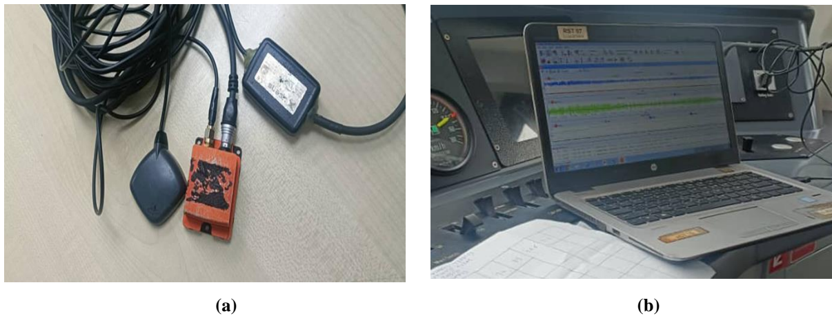
Fig. 4 Train Swaying Measurement tools (a) The sensor used (b) Measurement Process from Software
