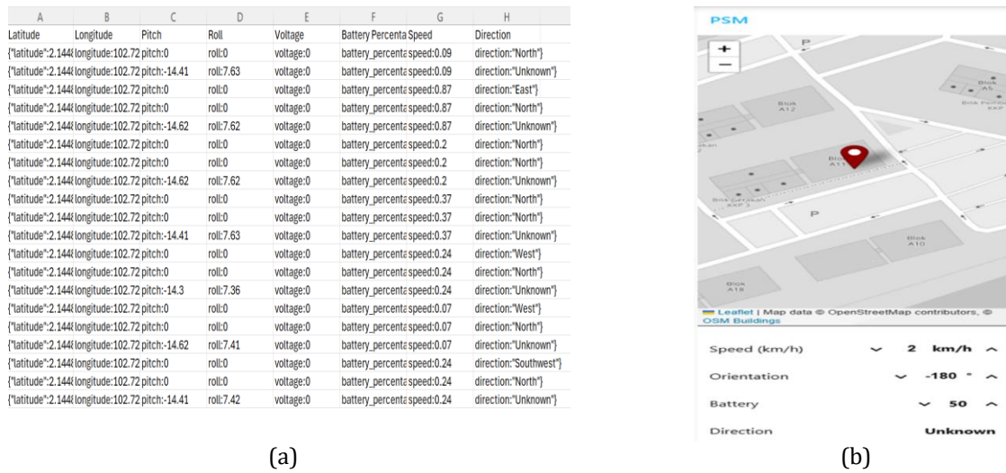
Fig. 6: Data Uploaded to Excel using MQTT Protocol (a); Node-RED Dashboard (b)
