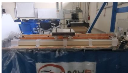
Figure 1.2: The Sliding TMD on the TMD Platform
