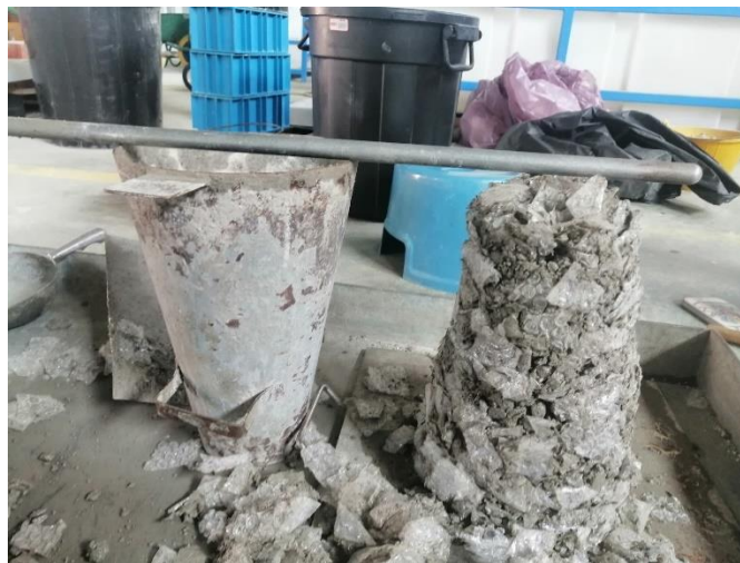
Figure 4.1: Zero Slump for 5% replacement LDPE aggregate
