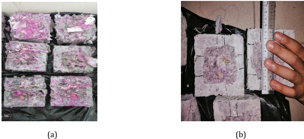
Figure 4.3: Point carbonation depth (dk point) measurement (a) spray with a fine mist of 1 percent phenolphthalein (b) Each points on each exposed concrete were measured
