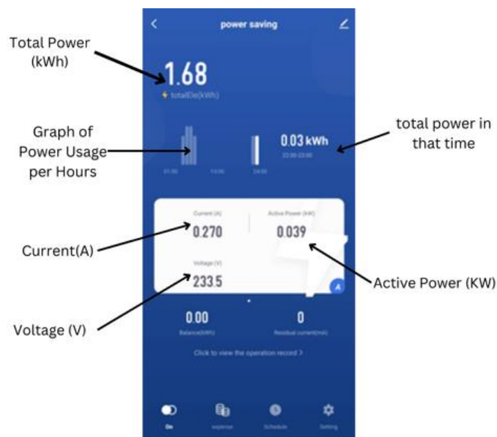
Figure Error! No text of specified style in document..5 list data shown on main interface
