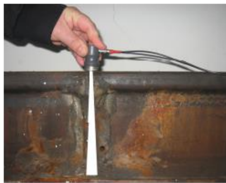
Fig. 2.4 UT testing on rail
