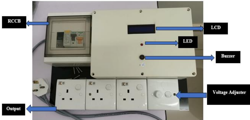
Fig. 8: Actual structure of the prototype
