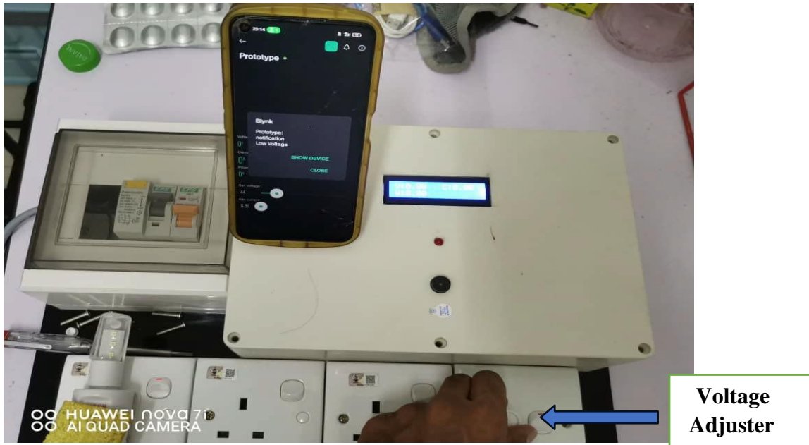
Fig. 10: Adjust voltage to create low voltage or high current situation
