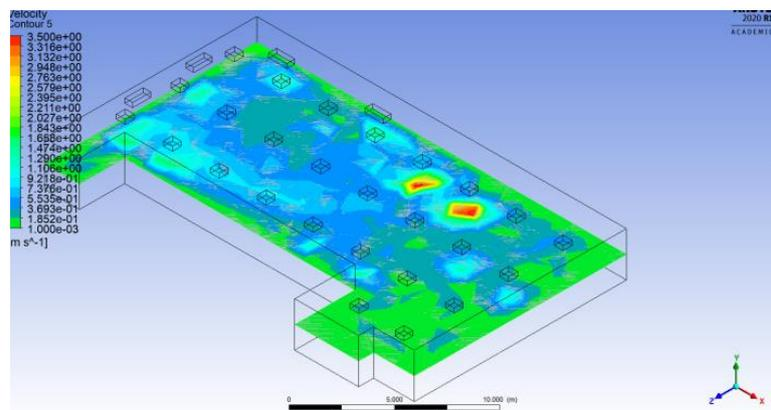
Figure 12: Velocity distribution from XZ view
