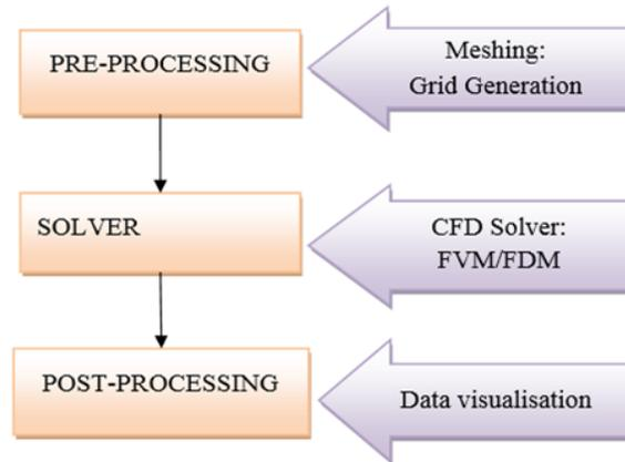
**Figure 4: Basic Process in simulation**
