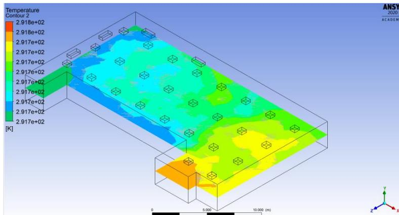
**Figure 10: Temperature distribution from XZ view**
