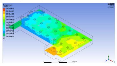
Figure 10: Temperature distribution from XZ view
