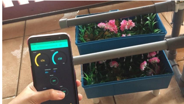
Figure 9: Both solenoid valves open and pump water to plant 1 and plant 2
