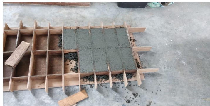
Figure 3: Mixture of perlite by percentage inside mould brick
