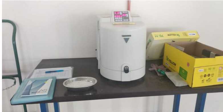
Figure 2: Planetary ball mill machine grinding Perlite to small particle
