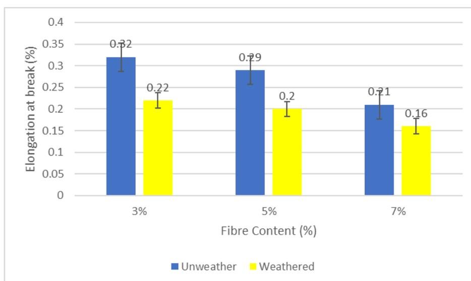
**Figure 11:** Elongation at break of silane treated bamboo fibre reinforced PLA/HDPE composites before and after natural weathering
