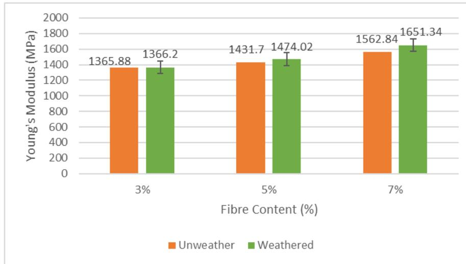
**Figure 7:** Young's Modulus of untreated bamboo fibre reinforced PLA/HDPE composites before and after natural weathering
