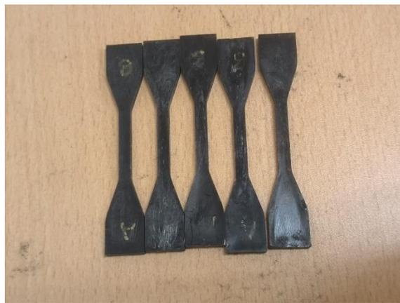
Figure 12: Specimens after exposure to natural weather
