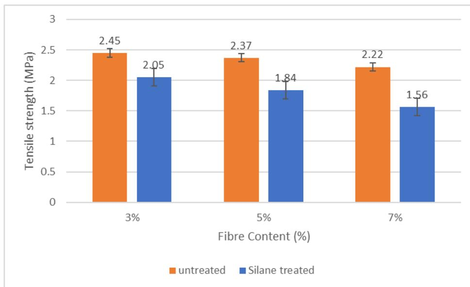
**Figure 3:** Comparison on untreated and silane treated of bamboo fibre reinforced PLA/HDPE composites in term of Tensile Strength
