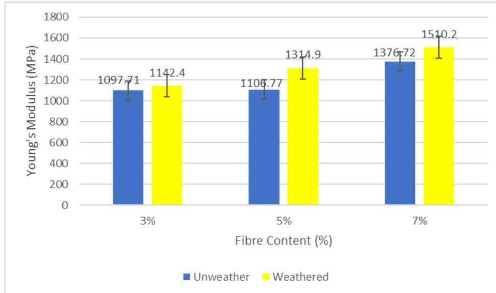
**Figure 10:** Young's Modulus of silane treated bamboo fibre reinforced PLA/HDPE composites before and after natural weathering
