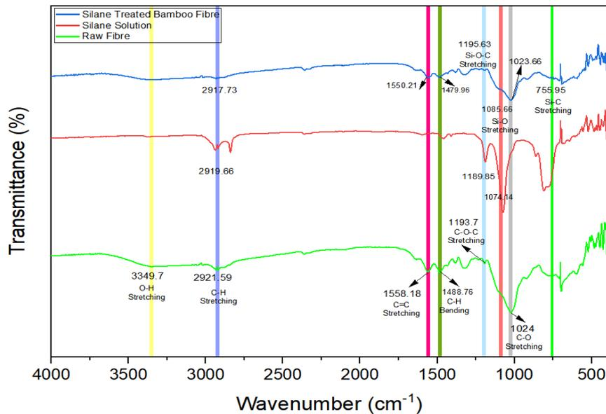
**Figure 2:** FTIR of untreated bamboo fibre, 3-aminopropyltriethoxysilane and silane treated bamboo fibre
