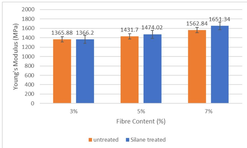
**Figure 4:** Comparison on untreated and silane treated of bamboo fibre reinforced PLA/HDPE composites in term of Young's Modulus
