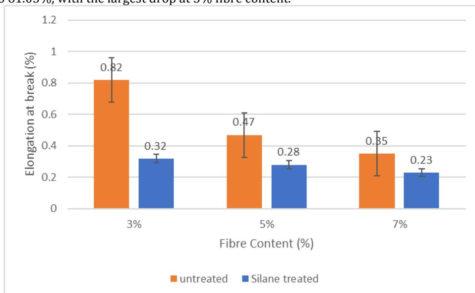
**Figure 5:** Comparison on untreated and silane treated of bamboo fibre reinforced PLA/HDPE composites in term of elongation at break
