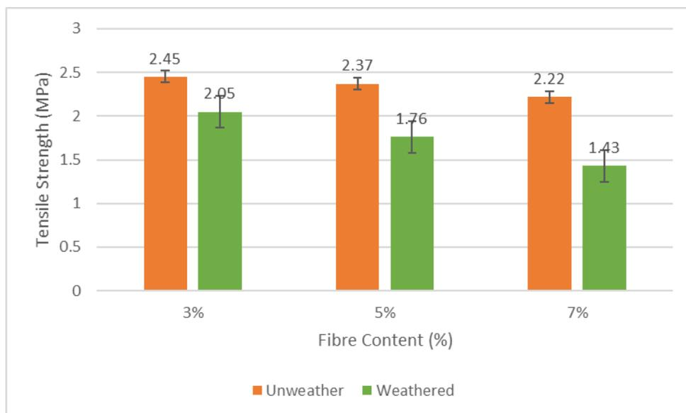
**Figure 6:** Tensile strength of untreated bamboo fibre reinforced PLA/HDPE composites before and after natural weathering.
