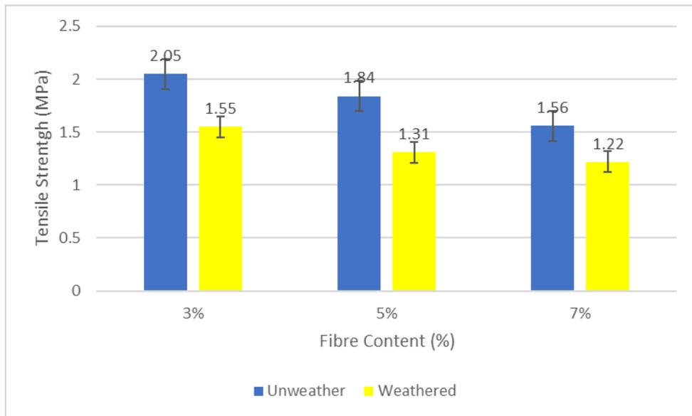
**Figure 9:** Tensile strength of silane treated bamboo fibre reinforced PLA/HDPE composites before and after natural weathering
