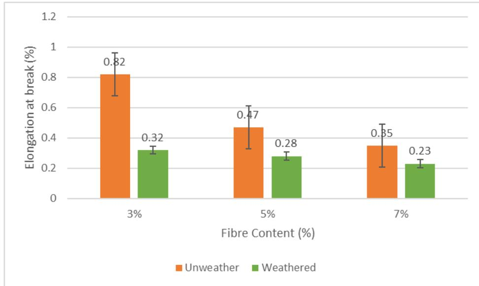
**Figure 8:** Elongation at break of untreated bamboo fibre reinforced PLA/HDPE composites before and after natural weathering
