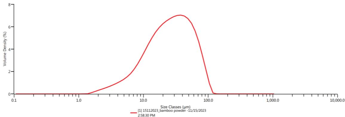
**Figure 1:** Particle size distribution of bamboo fibre
