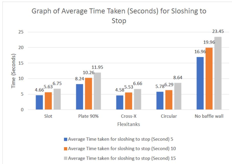
Fig 7 Graph of Average Time Taken (Seconds) for Sloshing to Stop
