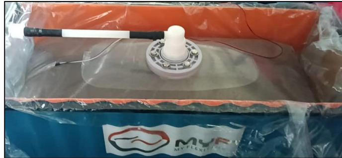
**Fig. 3** *Downscaled Flexitank setup*
