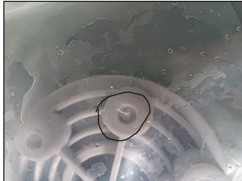
Fig 6 Tear damage (Cross-X)
