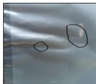
**Fig 5.** *Minor damage downscaled flexitank*
