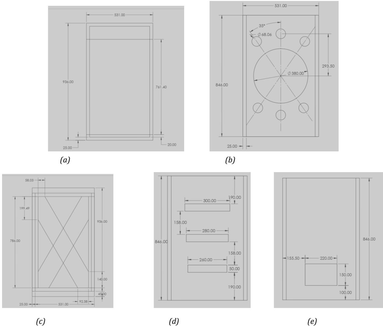
Fig 2. Horizontal Baffle Wall Dimension
