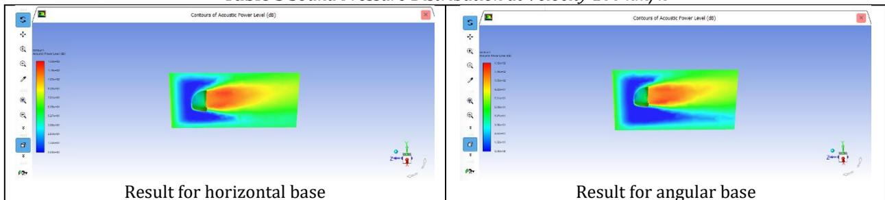
**Table 4** Sound Pressure Distribution at Velocity 120 km/h
