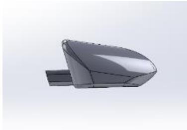
**Fig. 1** Side Mirror Base Model Horizontal in SolidWorks
