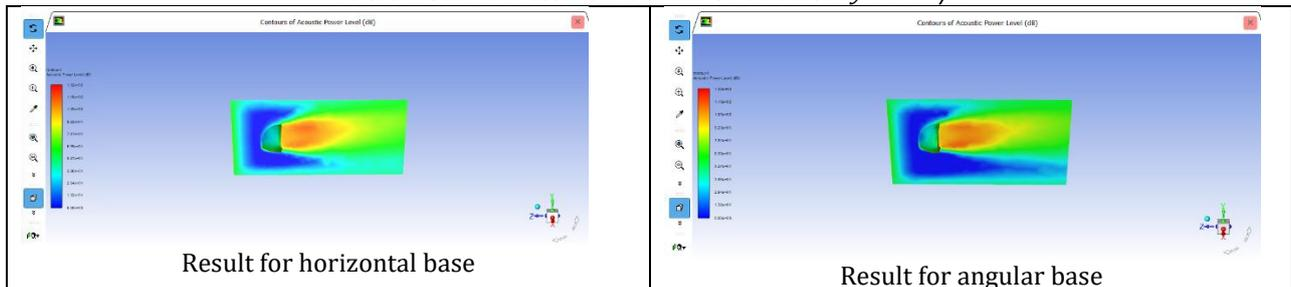
**Table 3** Sound Pressure Distribution at Velocity 100 km/h
