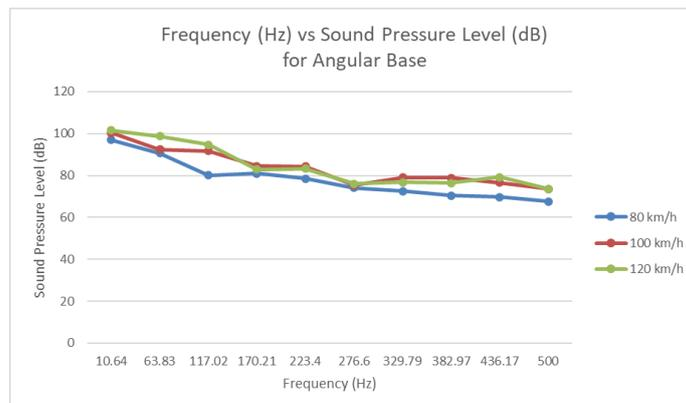
**Fig. 6** Sound Pressure Level (dB) vs Frequency (Hz) for angular base
