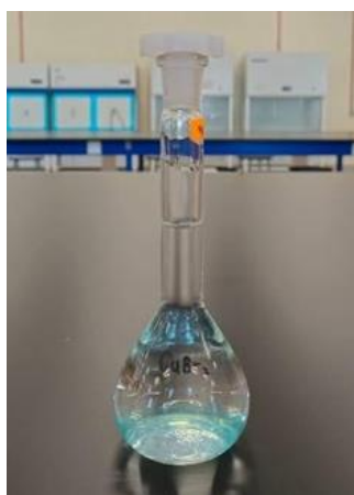
Figure 1: Light blue coloured solution of \text{CuBr}_2 in a volumetric flask
