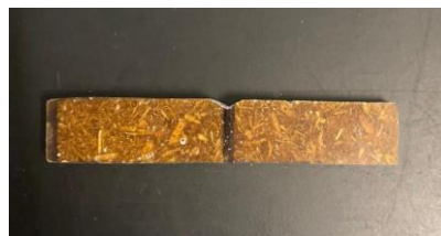
Fig. 5 Sugarcane bagasse fibre composite specimen for the impact test
