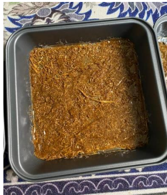
Fig. 2 Fabricate the mixture of sugarcane bagasse fibre with resin and hardener
