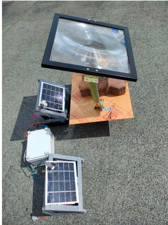
Fig. 12 The setup for Fresnel lens distance at 33 cm above solar panel
