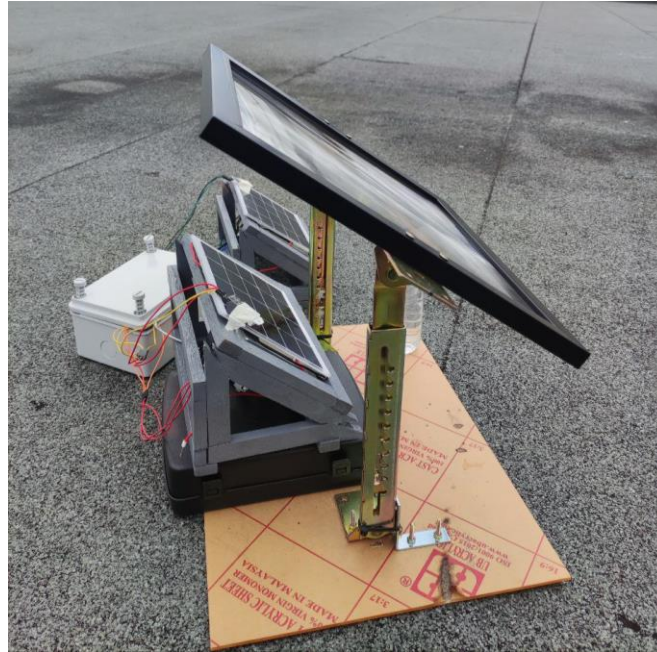
Fig. 9 The setup for Fresnel lens distance at 16.5 cm above solar panel
