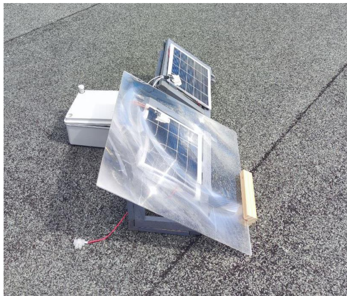
Fig. 6 The setup for Fresnel lens distance at 0 cm on the solar panel
