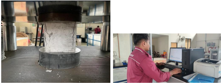
Fig. 2.1 Compressive Strength Test (a) Cube has been compressed (b) Collecting Data
