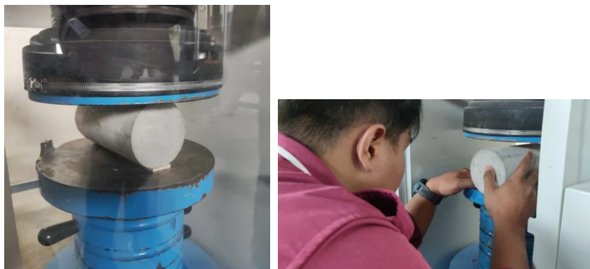
Fig 2.2 Tensile Strength Test (a) Sample being compressed for Tensile Strength (b) Retrieved sample.
