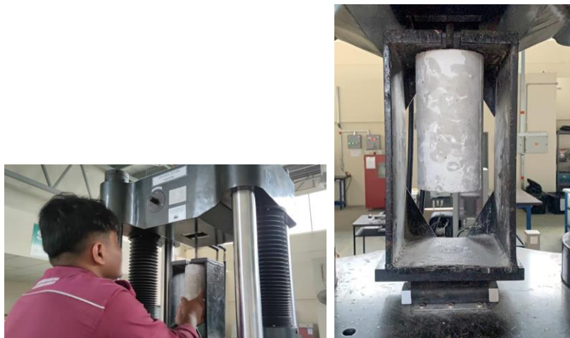
Fig 2.3 Pull Out Test (a) Preparation sample for testing (b) Sample being tested
