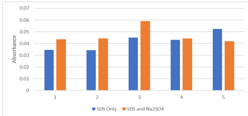
Fig. 5: Comparison graph for absorbance value between sample that contains only SDS and mixture of SDS and \text{Na}_2\text{SO}_4
