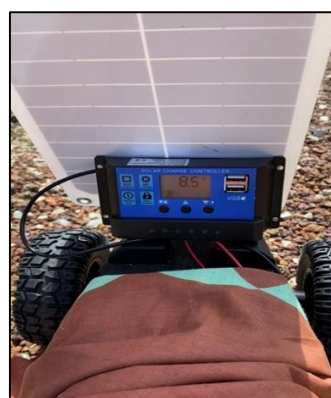
Figure 10: The Connections of Solar Charge Control
