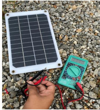
Figure 8: Measure the output voltage from solar panel.
