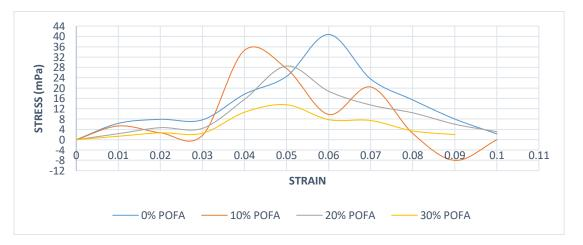
Figure 2: Relationship of Stress and strain on concrete cube containing 0.0 % POFA, 10.0 % POFA, 20.0 % POFA and 30.0 % POFA
