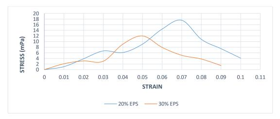
Figure 3: Relationship of Stress and strain on concrete cube containing 20.0 % Modified EPS and 30.0 % Modified EPS
