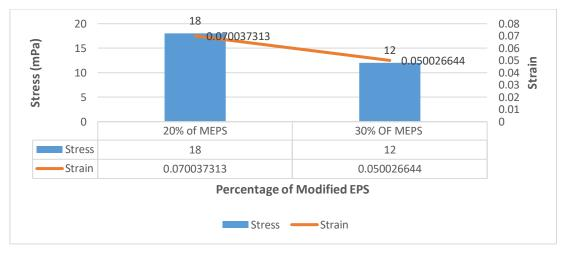
Figure 5: Highest Value of Stress and Strain on concrete cube containing 20.0 % Modified EPS and 30.0 % Modified EPS
