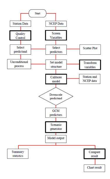
Figure 2: Schematic diagram of SDSM [13], [18]
