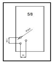
Figure 3: the dimensional for 16.6mm diameter of tube. [5]
