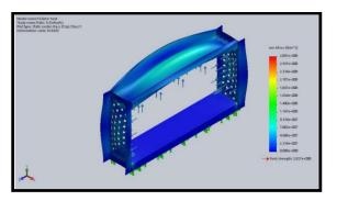
Figure 27: von mises stress value for 16.6 mm body frame heat exchanges for simulation
