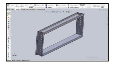
Figure 12: the holes tube condition if the total length is 1000 mm, total wide is 94 mm, and total height is 302 mm
