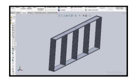
Figure 15: the holes tube condition if the total length is 4000 mm, total wide is 270 mm, total height is 1318 mm
