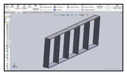
Figure 16: the holes tube condition if the total length is 5000 mm, total wide is 314 mm, and total height is 1598 mm
