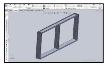
Figure 13: the holes tube condition if the total and total length is 2000 mm, total wide is 138 mm, and total height is 709 mm.
