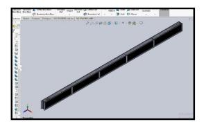
Figure 21: 1995pcs of fin plate, if the total length is 5000 mm, total wide is 314 mm, and total height is 1598 mm
