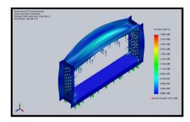
Figure 25: von mises stress value for 10.1 mm body frame heat exchanges for simulation
