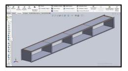
Figure 7: the number of center frame is 3pcs if the total length is 4000 mm
