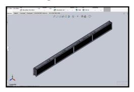
Figure 20: 1595pcs of fin plate, if the total length is 4000 mm, total wide is 270 mm, and and total height is 1318 mm
