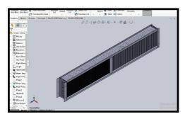
Figure 18: 8.5pcs of fin plate if the total length is 2000 mm, total wide is 138 mm, and total height is 709 mm
