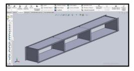
Figure 6: the number of center frame is 2pcs if the total length is 3000 mm
