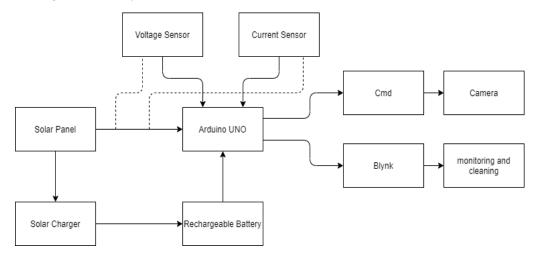
Figure 6: Block Diagram of robotic device for cleaning and monitoring photovoltaic panel arrays
