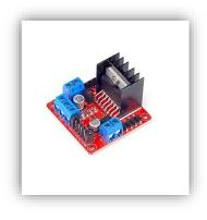
Figure 14: L298N Motor Driver Module
