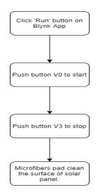
Figure 3: Flow diagram of controlling system
