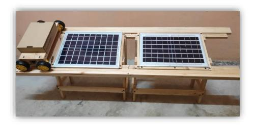
Figure 17: Solar panel with Cleaning Robot
