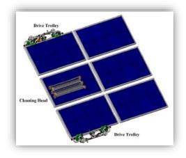
Figure 2: PVCleaner Robot V1.0
