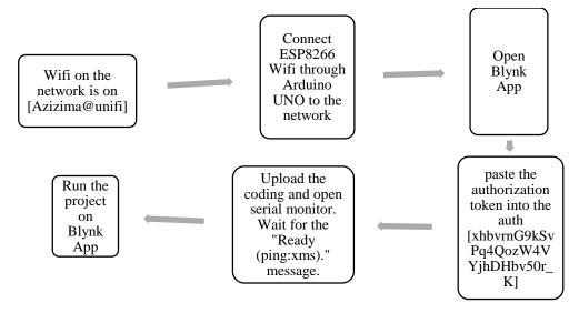
**Figure 4: Flow of Blynk Connection**
