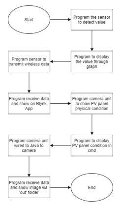
Figure 5: Monitoring Design Flowchart
