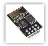
Figure 13: ESP8266 Wi-fi Shield
