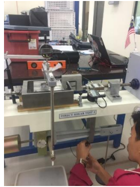
Figure 4: Direct Shear Test for SCE
