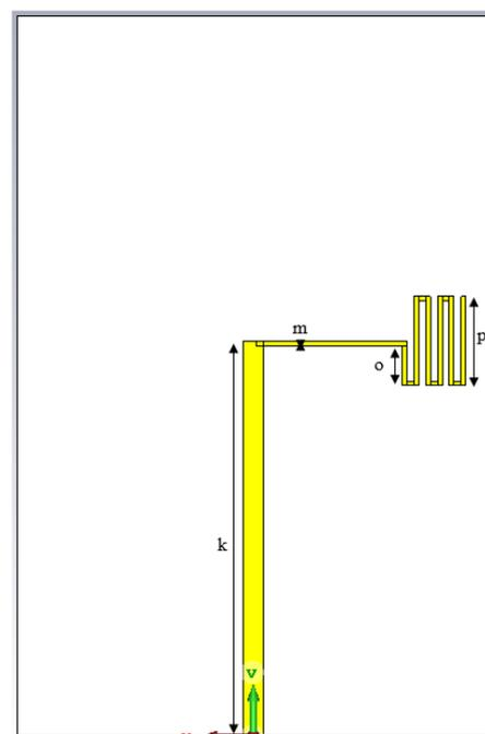
**Figure 5: Back view of the antenna with meander-line.**
