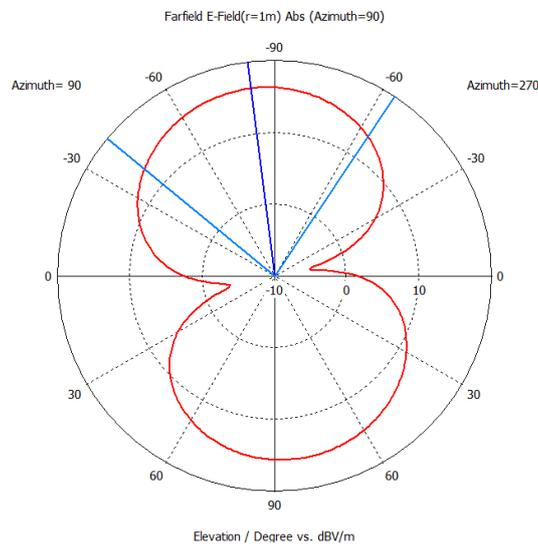
**Figure 9: Simulated radiation pattern with meander-line.**
