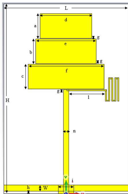
**Figure 4: Front view of the antenna with meander-line.**
