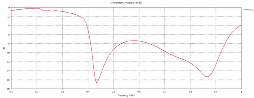
**Figure 6: Return loss of the antenna.**
