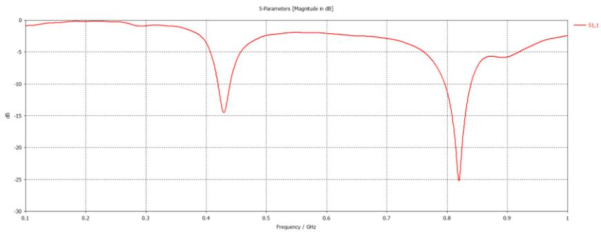
**Figure 7: Return loss results of the antenna with meander-line.**
