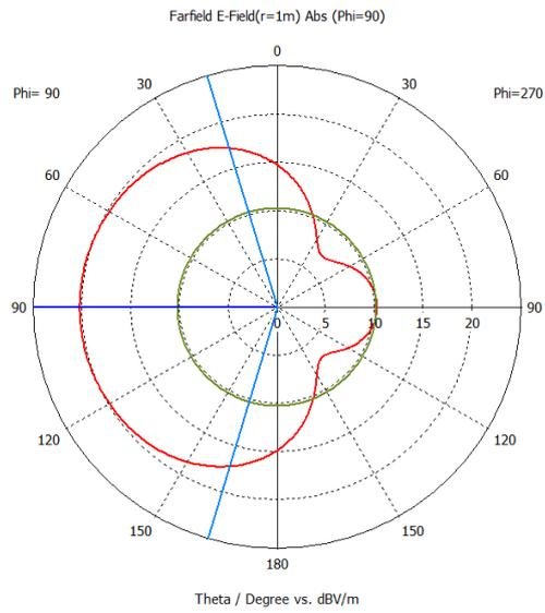
**Figure 8: Simulated radiation pattern for 0.433GHz**
