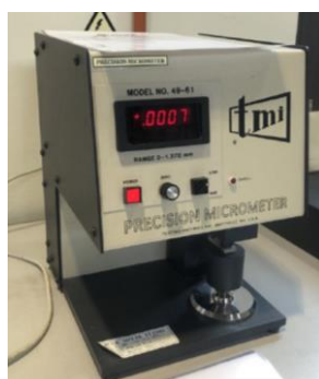
Figure 4: Precision Micrometer (Model No 46-6, Amityville N.Y. U.S.A.)
