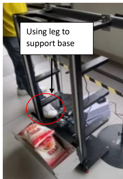
Figure 8: Base need support by leg
