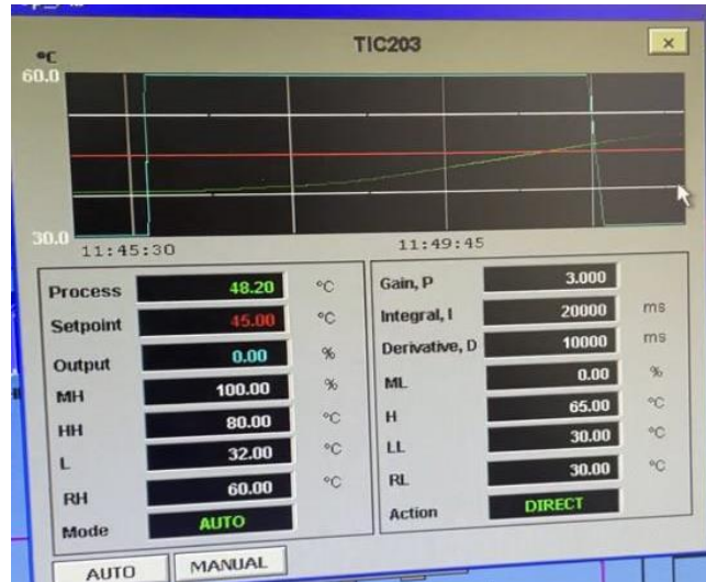
Figure 2: Default setting in DCS of the parameters proportional integral derivative PID and result of the process heating temperature at vessel VE203
