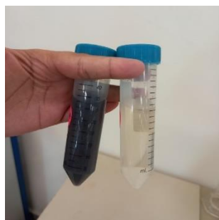
Figure 6: The colour of textile dye wastewater before and after the filtration
