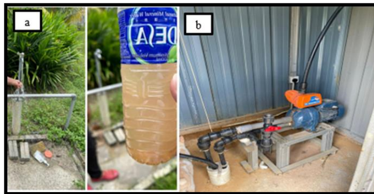
Figure 2 & 3 : Groundwater sample collection from (a) faucet connected to the (b) pump of tubewell.
