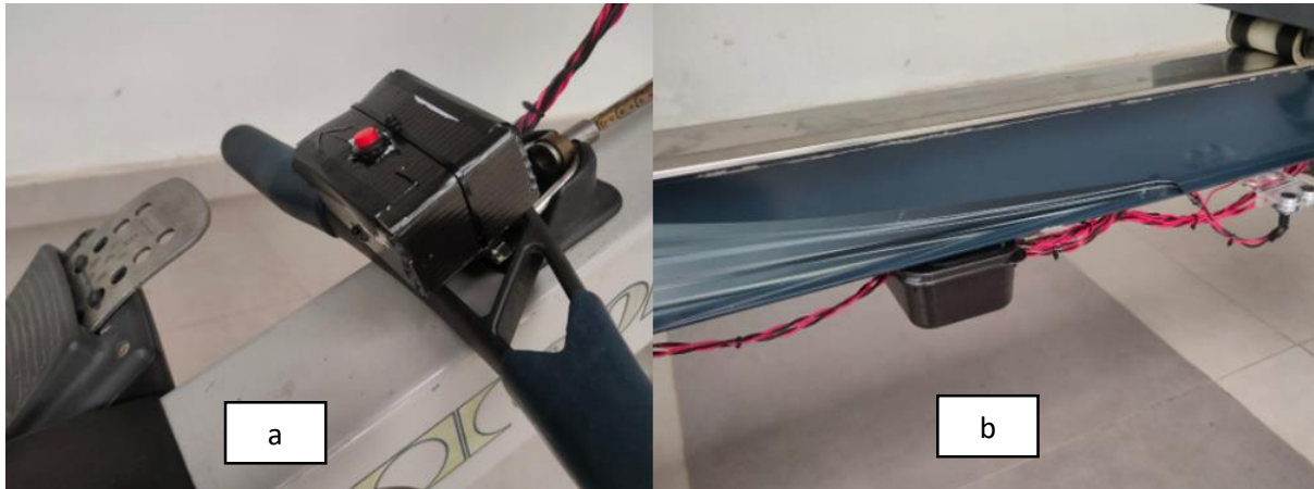
Figure 7: (a) Device on the handle rowing machine and (b) microcontroller box
