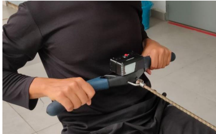
Figure 9: Handlebar that already install with handle box have been pull
