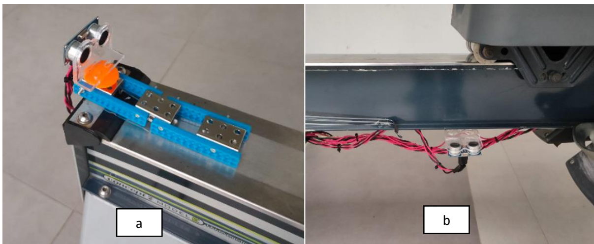
Figure 8: (a) Ultrasonic sensor for the back (b) Ultrasonic sensor for the leg
