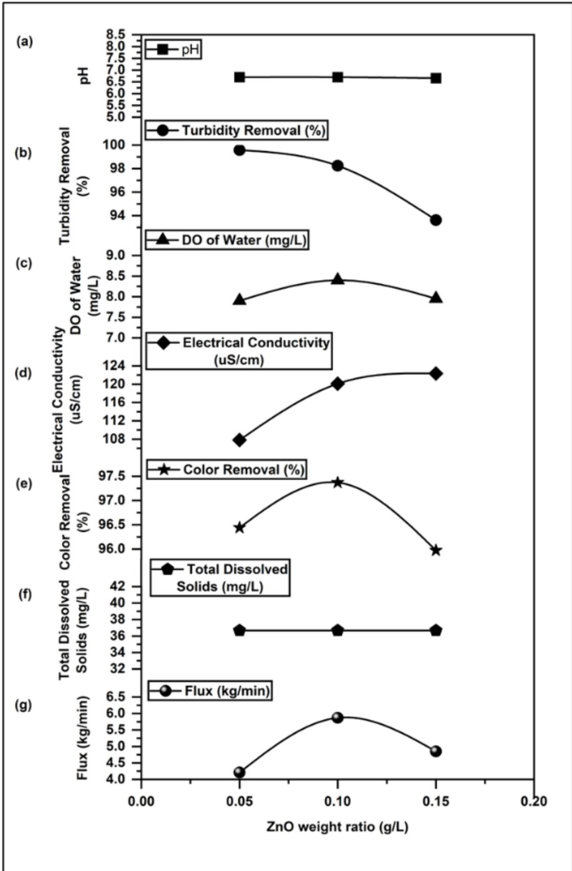
Figure 4: Effect of catalysts (ZnO) loading with membrane (a) pH, (b) Turbidity, (c) DO, (d) Electrical conductivity, (e) Color, (f) TDS, and (f) Flux
