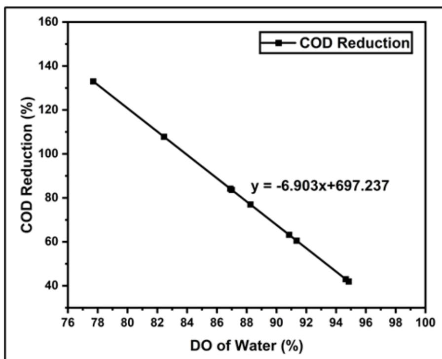
Figure 6: Prediction chart for on-site monitoring of COD based on DO
