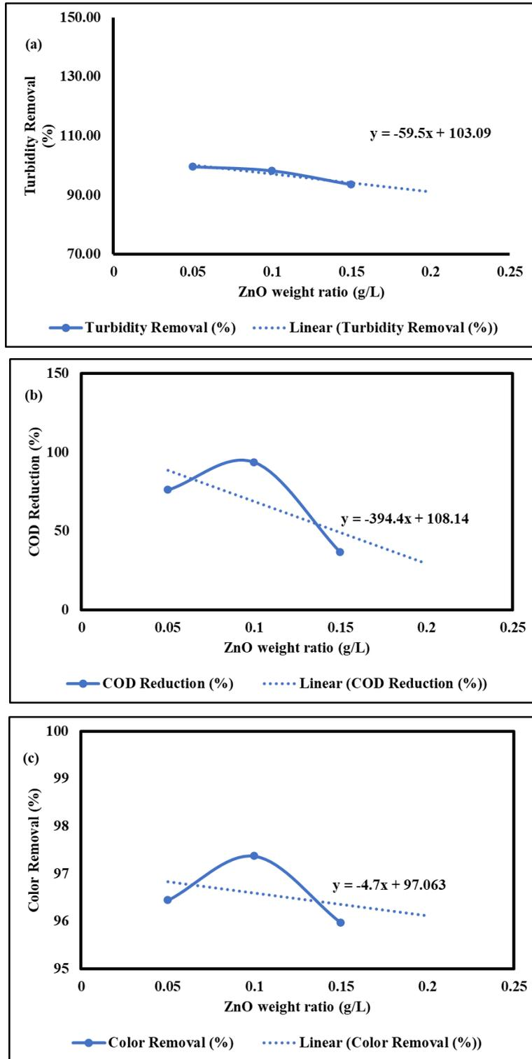
Figure 5: Kinetic model of MPR's performance (a) Turbidity, (b) COD, (c) Color
