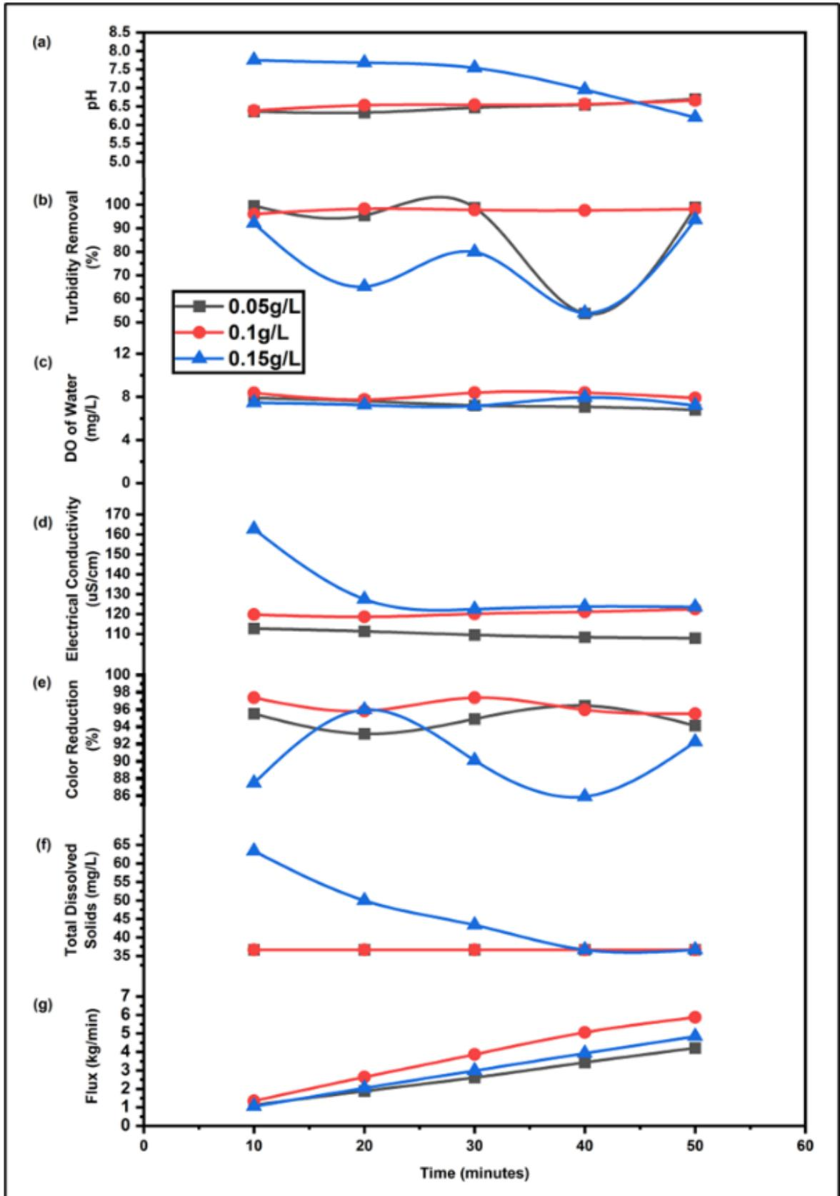
Figure 3: Correlation of reaction time on photocatalytic reactor with hollow fiber membrane performance (a) pH, (b) Turbidity, (c) DO, (d) Electrical conductivity, (e) Color, (f) TDS, and (f) Flux
