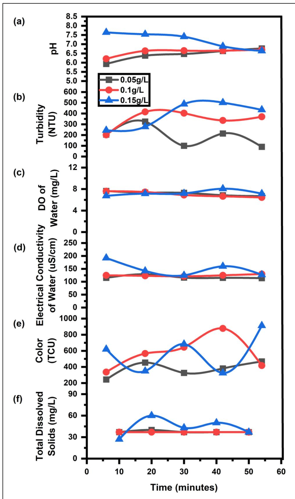
Figure 2: Correlation of reaction time at photocatalytic reactor performance (a) pH, (b) Turbidity, (c) DO, (d) Electrical conductivity, (e) Color, (f) TDS
