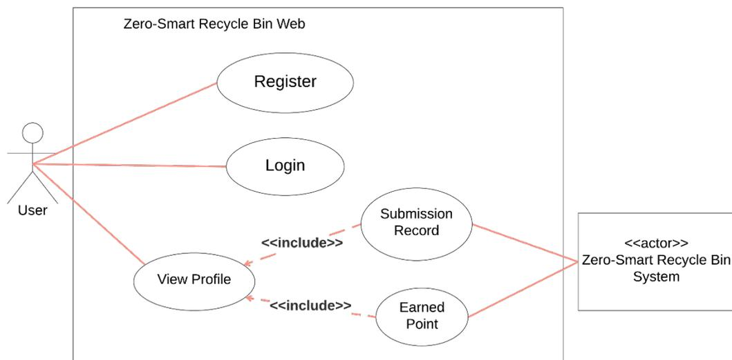
**Figure 2 : Use Case Diagram of the Zero-Smart Recycle Bin User Web Application**
