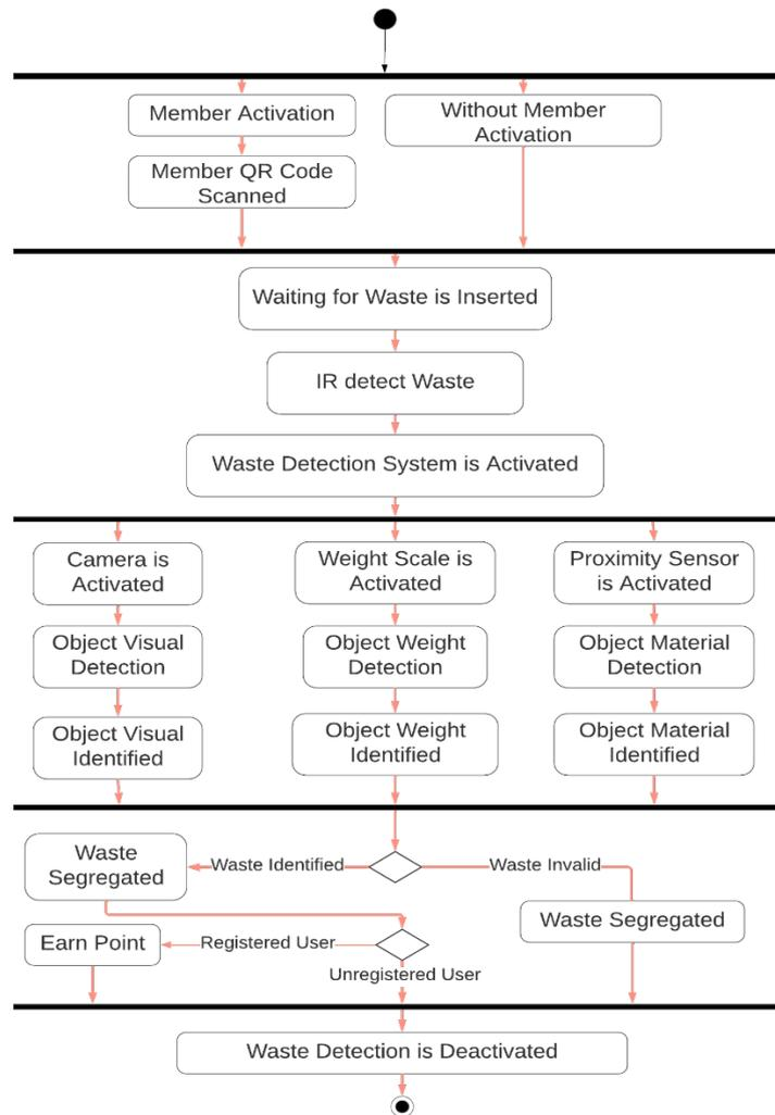
**Figure 1: Activity Diagram of the Zero-Smart Recycle Bin**
