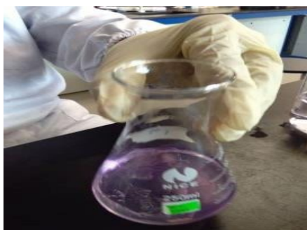
Figure 3: The colour of ethanol: phenolphthalein changes after titration with KOH to determine free acid content in S1 and S2
