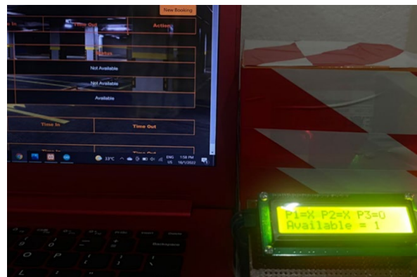
Figure 11: The Status of the LCD and Website when Two Slots are Occupied
