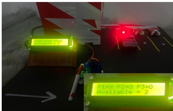
Figure 6: LCD displays the Status of the Car Park when it is Empty
