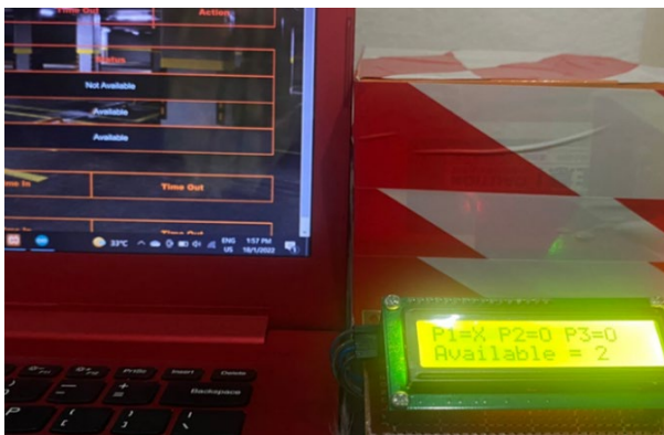
Figure 10: The Status of the Webpage and LCD when One Slot is Occupied
