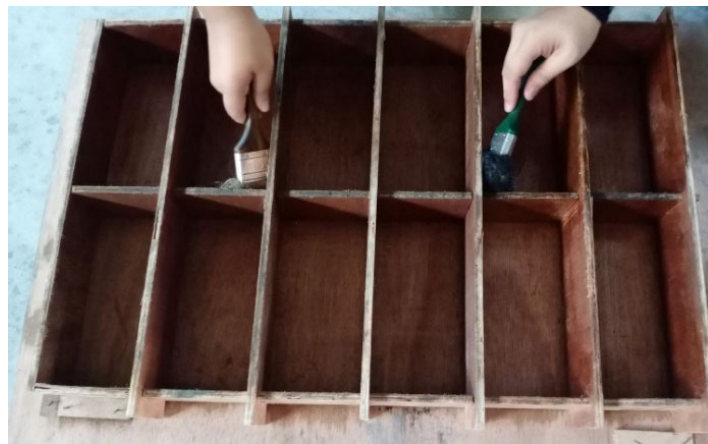
Figure 2: The mould used to cast control bricks and Eco-Bricks
