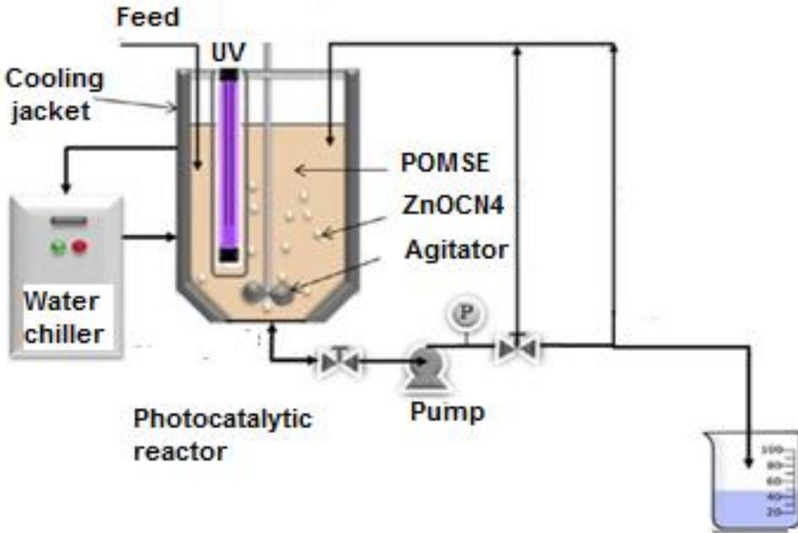
**Figure 1 : Schematic diagram of a laboratory-scale photocatalytic reactor**
