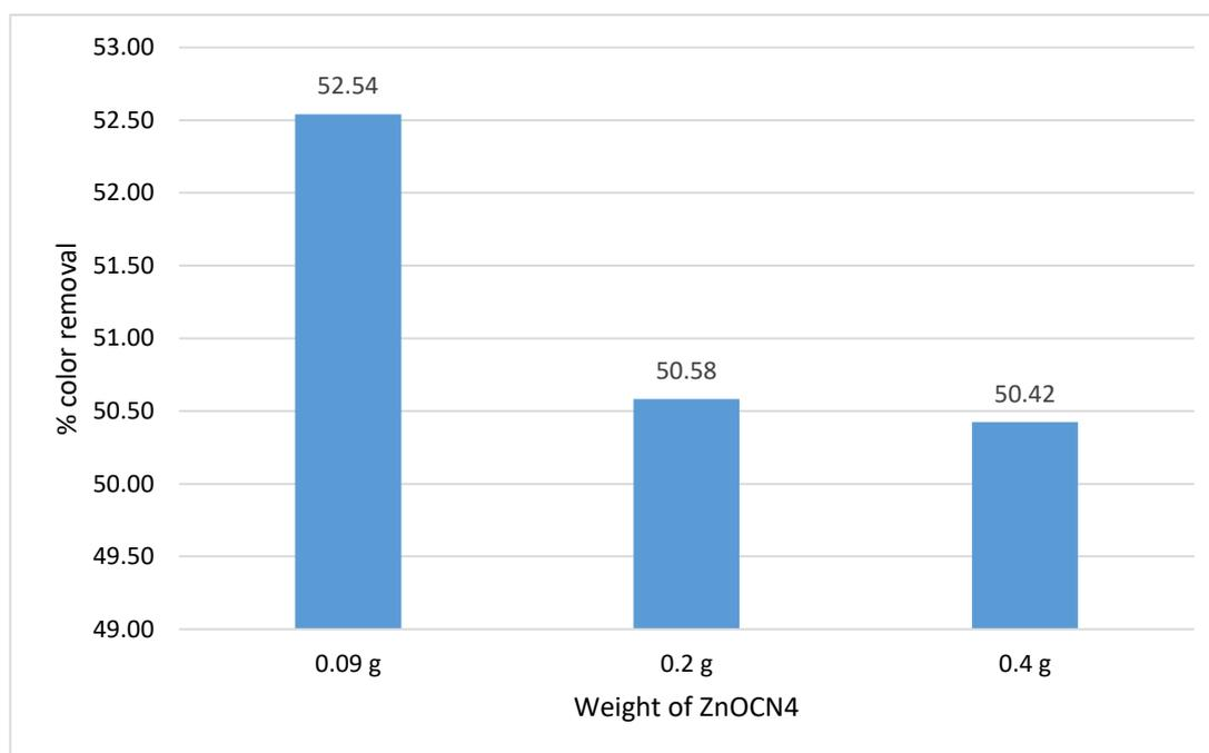
**Figure 2: % color removal of POMSE at various weight of ZnOCN4**
