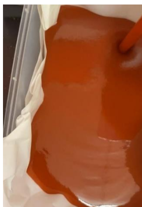
Figure 1: Mixture of NaOH solution with waste cooking oil.
