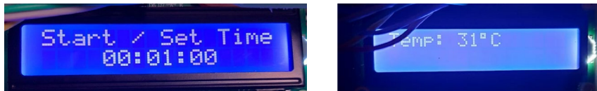
Figure 6: LCD to display the start or time setting for heating process and temperature inside lunchbox
